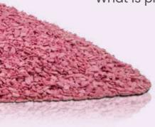
Pressure granulation is a process changing the form of powdered products into granulate. The powders, under the high pressure, are given the form of fine grains to improve their technological features and widen the application range.
